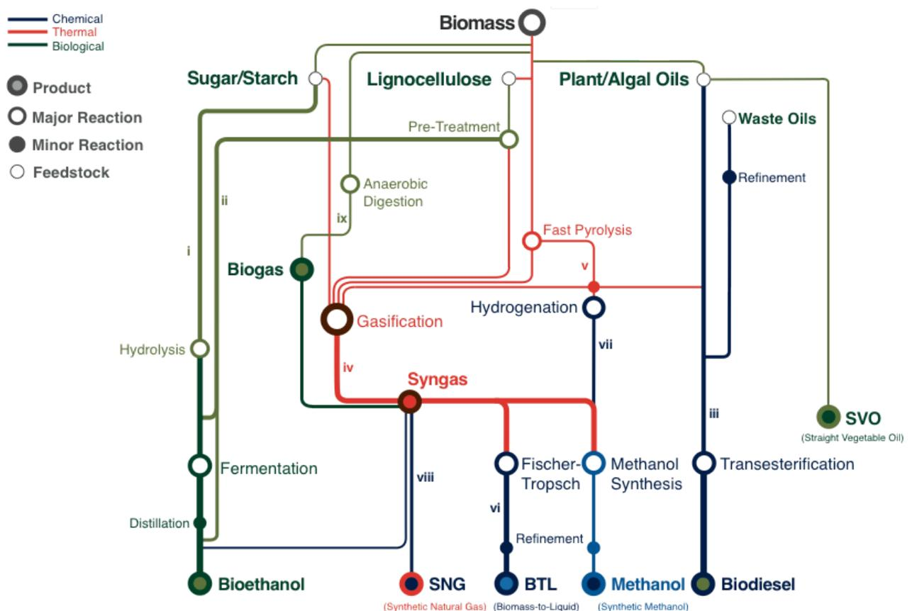
Figure 1: *Biofuel Flow*. The multiple synthetic conversion routes of major biofuels produced from first and second-generation biomass feedstock. Roman numerals correspond to the conversion processes described in section 1.2.
