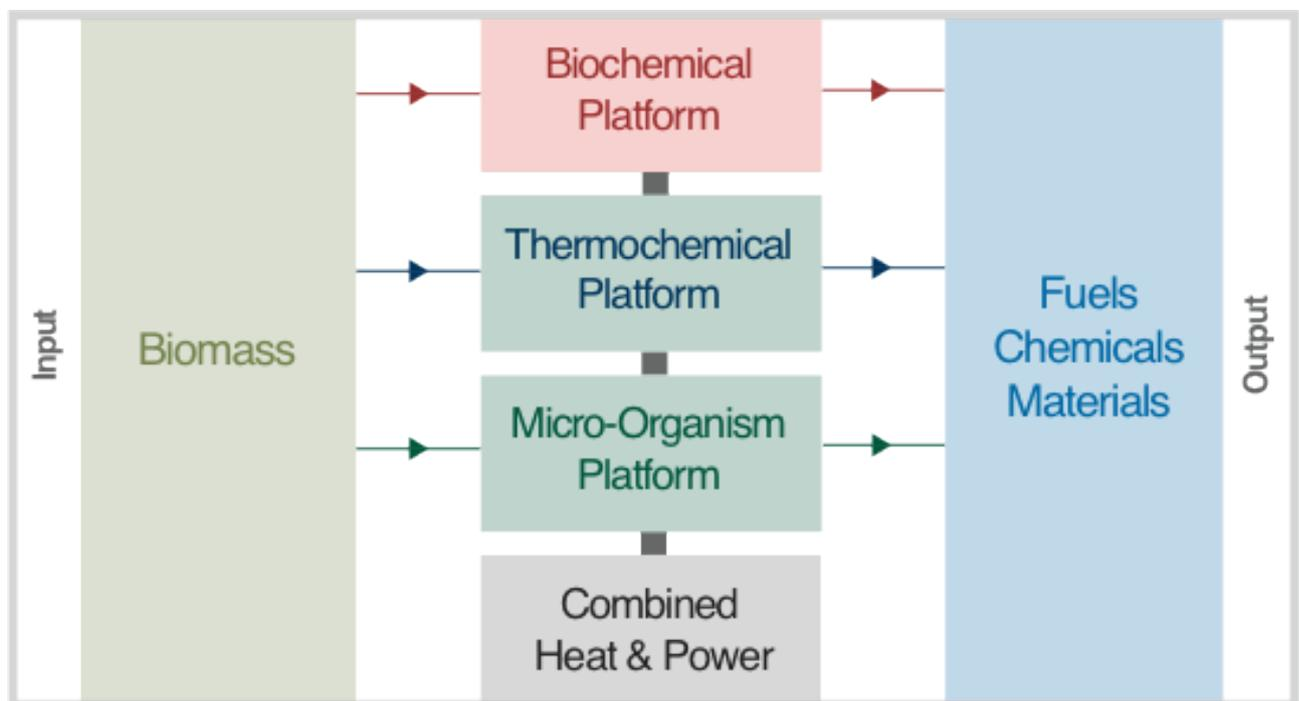
Figure 2: *The Biorefinery Concept*. A simple three “platform” concept adapted from a model devised by the National Renewable Energy Laboratory to include a microorganism platform. This concept demonstrates how any number of conversion processes can take place within one biorefinery, analogous to today’s oil refinery.
