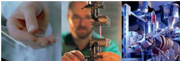
(left to right): Film made of modified starch, Testing mechanical properties, Compounding thermoplastics with cellulose man-made fibers, © Fraunhofer IAP.
