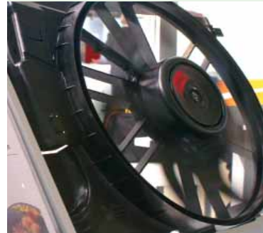
Motor engine cooling fan and housing module made from Nylon-5,10. Picture: BIOPRO/Bächtle. Prototype: Robert Bosch GmbH.
