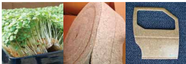
Left to right: Hemp fibre bounded with PLA-fiber a growth medium for spicy herbs, nonwoven hemp fibre mats, reinforced bio-composite. Pictures: Bodil Pallesen.
