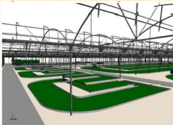
Fig. 25.- Detailed scheme of thin-layer cascade and improved raceway units to be installed
