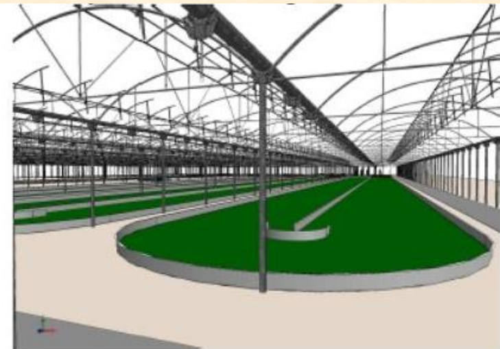
Fig. 25.- Detailed scheme of thin-layer cascade and improved raceway units to be installed
