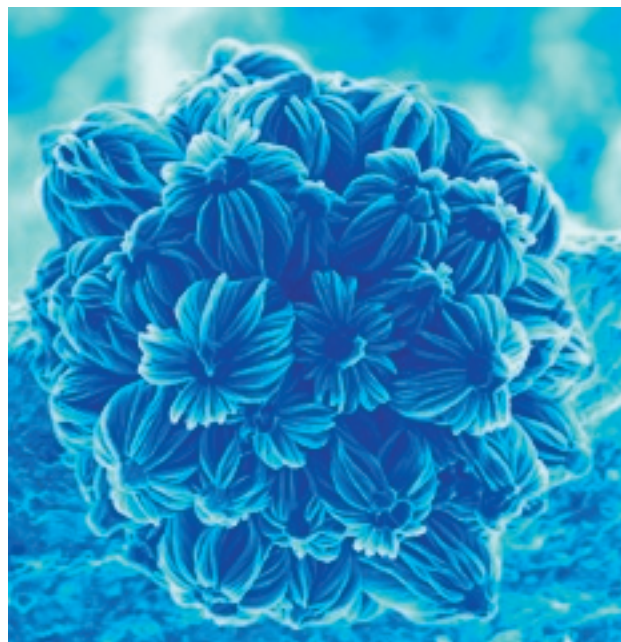
A 3-D nanomaterial grown from tiny droplets of a liquid metal on a silicon surface.
