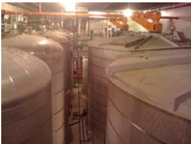
Figure 41. a) 35,000 Gal. Hydrolysis Reactors and b) 10T/D Pre-treatment Skid [ICM]
